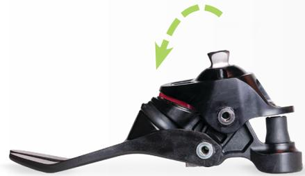
To ready the foot for a smooth toe-off, the Truststep's front bumper compresses to absorb impact and lift the heel. The rollover shape and contoured toes assist in forward propulsion.
