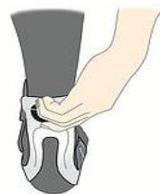
4. Turn the dial lock clockwise to adjust the AF SERVO to your foot shape.
